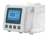
The extriCARE® 3600 Negative Pressure Wound Therapy (NPWT) device is a portable, battery powered pump designed for use in hospitals, wound care centers, and other medical facilities. The extriCARE® 3600, used in conjunction with our anatomically fitted line of wound dressings, may promote wound healing through the drainage and removal of wound exudates, infectious material, and tissue debris from the wound bed using continuous and/or intermittent negative pressure.
